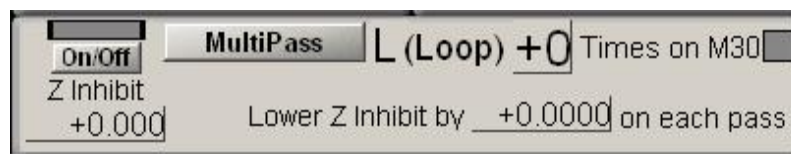
Figure 6.19 – Automatic Z control
